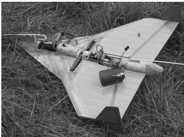
Fig. 4 A view of the MAV showing the batteries and avionics bays with the power plant controller and the data acquisition system (photo by Jarosław Hajduk).
